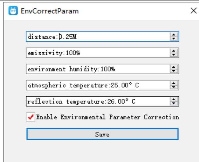
1. Reflected temperature: Infrared rays emitted by surrounding objects will be reflected by the target object.
