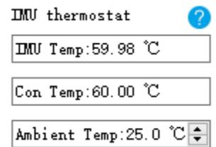
Before calibration, please input the environment temperature of your operating field, the software will start to calculate the target IMU constant temperature so that IMU can reach the temperature fast after powering on gimbal camera. The software is showing IMU temperature in real-time.
