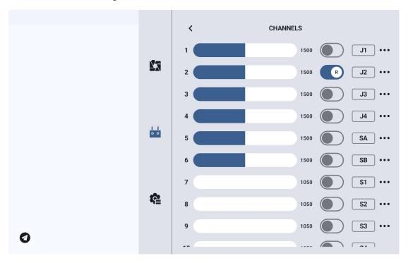
Select the target channel, then click the corresponding servo direction toggle switch to successfully set the servo to normal or reversed direction.
