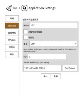
4. Select the configured "UDP" connection and click "Connect". When the progress bar at the top of the QGC interface starts moving, it indicates that the handheld ground station and the flight controller ground station software are attempting to establish telemetry communication. Once the connection is established, data communication will proceed normally.
