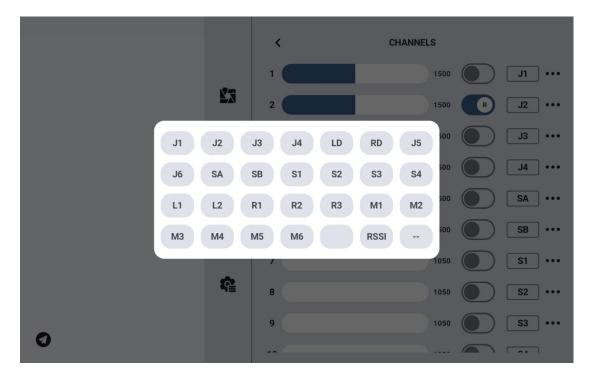
Select the target channel and click the channel mapping button. A switch list will pop up—choose the desired switch to successfully complete the connection.
