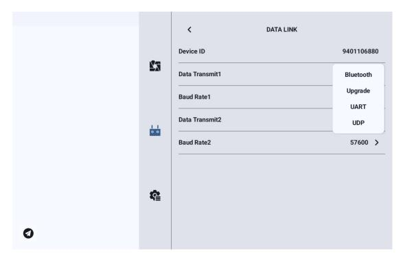
UART Serial Port: Data transmission communication is conducted via the built-in UART serial port of the ground station (developers can refer to the data transmission SDK documentation in Chapter 6 of this manual to develop support for this function on their own ground stations).
