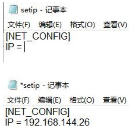
Then insert the SD card to the camera and restart the camera. After waiting for three to five minutes, the IP addresses will be flashed into the camera. Then we restart the camera again to finish changing IP addresses.
