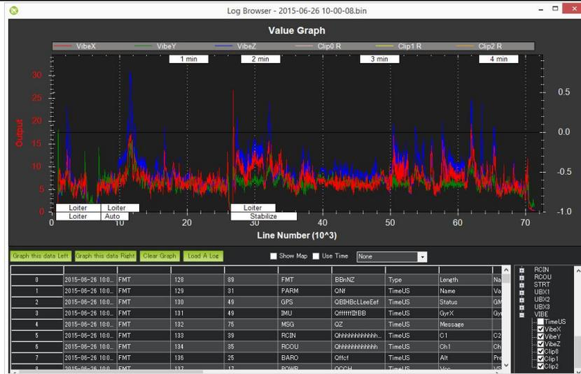
This is an example of a vehicle that had position estimate problems due to high vibrations.
