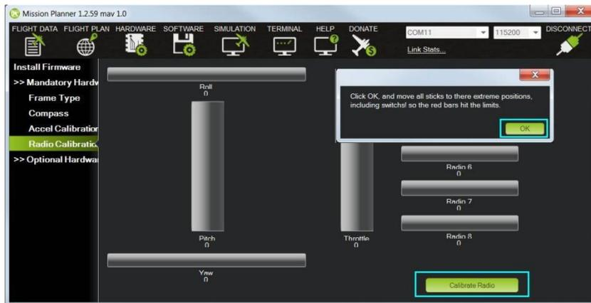
6. Move the transmitter's control sticks, knobs and switches to their limits. Red lines will appear across the calibration bars to show minimum and maximum values seen so far.
