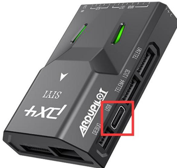
3. Run Mission Planner GCS, select the COM port drop-down in the upper-right corner of the window near the “Connect” button. Select “AUTO” or the specific port for your board. Set the Baud rate to “115200” as shown. Do not hit “Connect” just yet.
