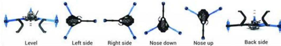
4. The vehicle must be kept still immediately after pressing the key for each step. This is more important than getting the angle exactly right, i.e., left being 90-deg to horizontal, etc. Except for the first “LEVEL”, the positions can be within 20 degrees of being exact. Being still in each position as you press the key is much more important.
