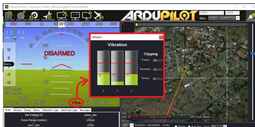
Vibration levels below 30m/s/s are normally acceptable. Levels above 30m/s/s may have problems and levels above 60m/s/s nearly always have problems with position or altitude hold.
