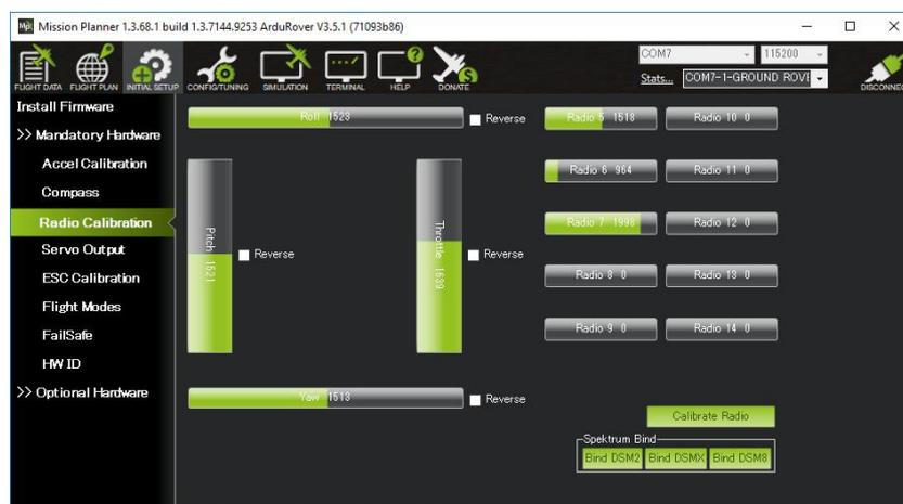
5. Click on the green “Calibrate Radio” button on the bottom right. Press “OK” when prompted to check the radio control equipment is on, battery is not connected, and propellers are not attached.
