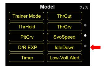
Idle Down function is designed for planes, helicopters, and other models powered by engines.
