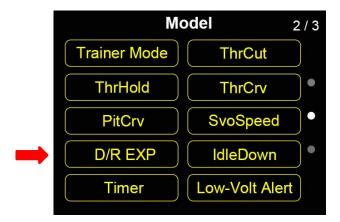
On three channels, Aileron / Elevator / Rudder, FT24 transmitter supports increasing / decreasing channel output value by operating a physical switch for better operating experience. Users can also preset three ratios for the channels.
