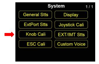
Knob Calibration help maintain both knobs' output accuracy. Calibration is required when the knobs stay out of their middle position (channel value is not 0) or do not reach the maximum / minimum position.
