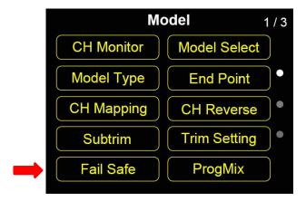
After binding FT24 transmitter to its receiver, do not forget to configure Fail-Safe and turn on the function. Then if your transmitter lost control to receiver, Fail-Safe function runs automatically and immediately to protect your model from a crash.
