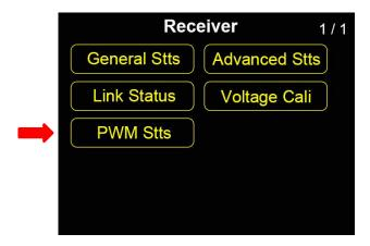
Users can re-define all 8 PWM channels on FR receiver through PWM settings. In default, PWM channels 1 to 8 are mapped with transmitter channel 1 to 8. They are free to be mapped with all 16 transmitter channels.
