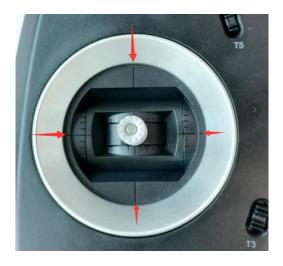
5. FT24 Transmitter starts detecting middle positions automatically, do not touch the joysticks while you are waiting;
