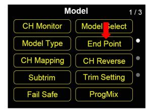
"End Point" page helps users configure channel output value and output limit.
