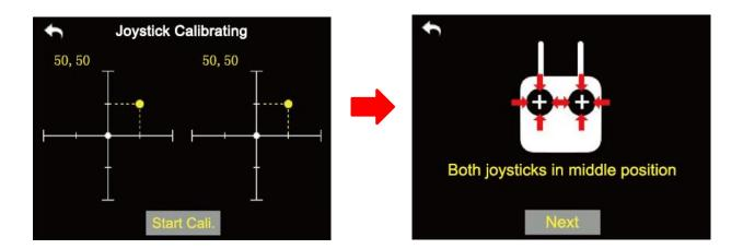
4. Hold / Adjust both joysticks to make them stay in middle positions (when joystick's tick mark aligns with the transmitter's tick mark), then enter "Next".
