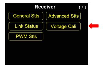
Before using FR receiver, SIYI suggests that user should manually calibrate receiver RX Voltage and PWR Voltage once.
