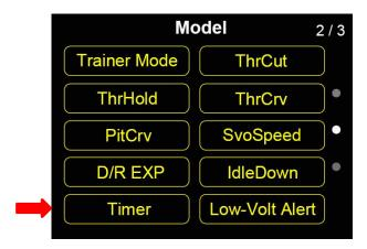
FT24 transmitter supports up to 2 Timers which can be used simultaneously.
