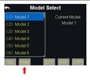
2. Input a new name for the model by using the virtual keyboard, then "yes" to finish.
