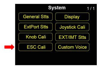
FT24 transmitter simplified ESC calibration process. Users just wire their ESC with FR receiver's PWM port 1 to 8, then follow what the transmitter guides in "ESC Calibration" page the steps below to do calibration.
