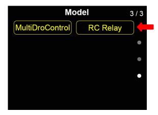
RC Relay function is designed for long range flight which can only be done by relay control between two FT24 transmitters.
