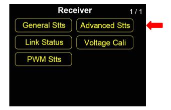
Advanced Settings is to setup baud rate for datalink/telemetry function. Range: 4800, 9600, 38400, 57600, 76800, 115200, 230400.
