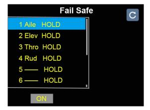
4. In Fail-Safe page, the function is default to be "OFF" and it displays "HOLD" in each channel. Under this configuration, if transmitter lost control to receiver, the receiver
