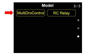
FT24 transmitter supports users to control up to three drones (receivers / aircrafts) simultaneously.
