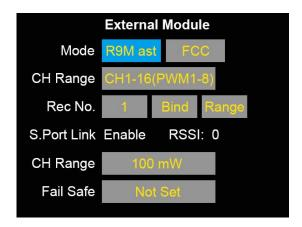
Plug R9M radio module into FT24 transmitter and switch the mode to "R9M ast", transmitter will start to communicate with R9M. And you can monitor information such as signal strength, S.BUS / PPM signals, etc.
