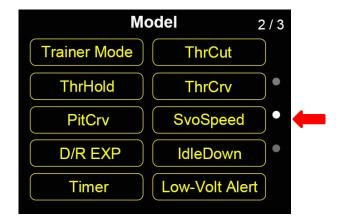
Servo speed function is designed to accomplish some special mission by adjust the changing ratio of an output channel. For example, it could be too fast to pack up or lay down landing gear in normal servo speed. So, we increase the channel's output ratio. Larger the value is, slower the channel outputs.
