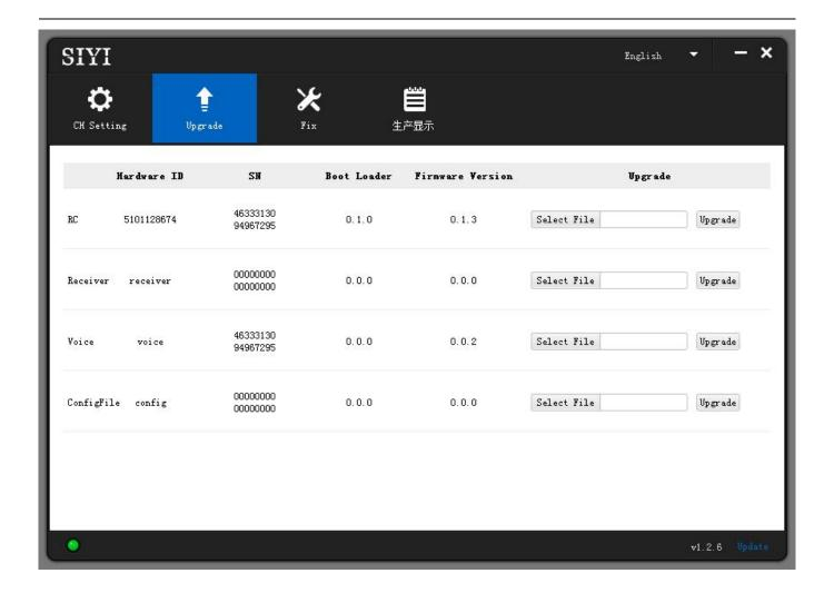
3. Upload the latest firmware files for FR / FR Mini receiver and click on "Upgrade". Then wait till the process is 100% finished.
