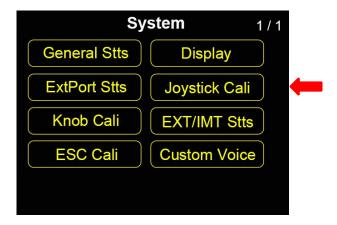
Joystick Calibration function help users calibrate both joysticks' middle position, especially when they don't stay in middle (Channel Output is not 0) or don't reach their maximum and minimum limits. Regular calibration helps maintain control accuracy of the joysticks.
