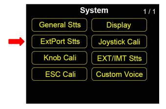
Expanding Ports function allows users to adjust FT24 transmitter outputting settings for supporting more external devices.
