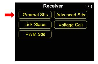
General Settings is to setup different signal modes for FR receiver, according to its different output mode (S.BUS, PPM, and PWM).
