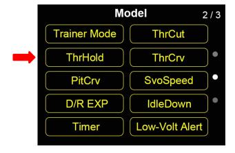
When Throttle Hold function is turned on, throttle channel is forced to output a fixed value. In this case, pushing on throttle stick does not output no value. Turn off the function to be back normal.
