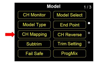
All 16 channels in FT24 transmitter can be mapped freely to joysticks, switches, buttons, and dials.
