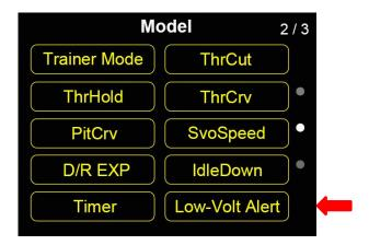
By using telemetry function, users can set a minimum voltage limit as safe level on FT24 transmitter, lower than which transmitter will send voice alert.
