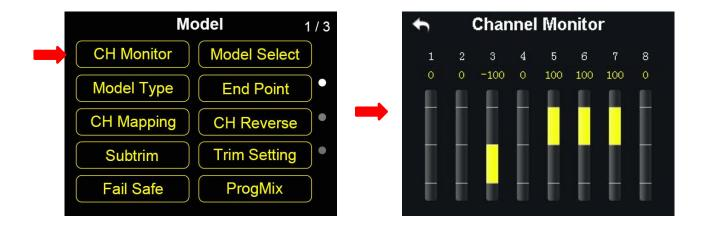
Channel Monitor page is for real-time monitoring and configuring output values of all 16 communicational channels.
