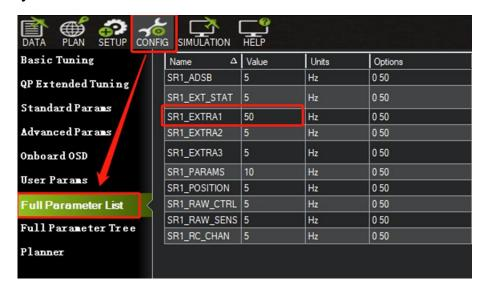
After configuration, it is necessary to "Write Parameters" and reboot the flight controller to take effect.
