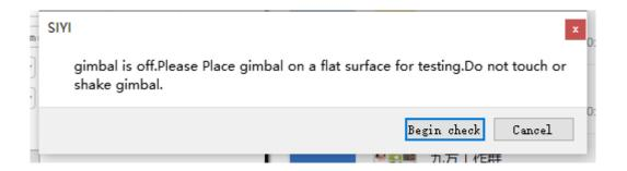
2. The PC assistant start to check IMU status automatically to determine if the gimbal should be calibrated.
