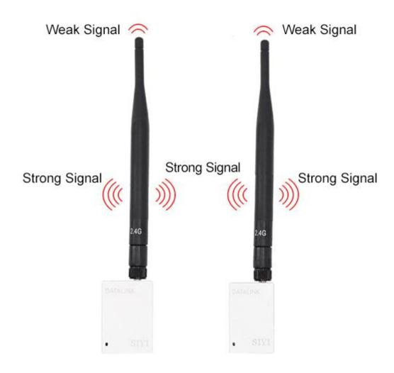
Mark: 2.4G Datalink has the best signal strength when the antennas are placed horizontally. Thus, please avoid pointing antennas' upper end straightly to your aircraft and do not fold the antennas.
